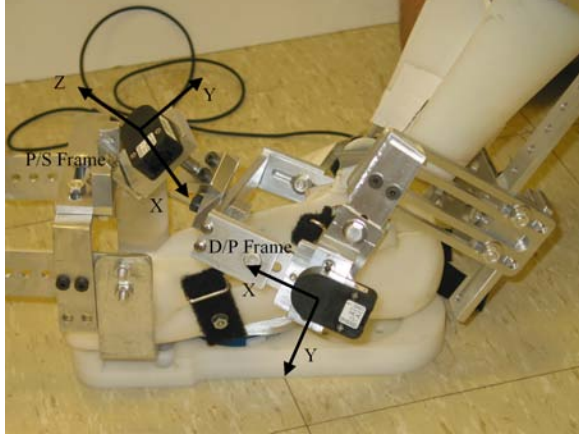
Fig. 5. Orientations of the D/P and P/S frame. This picture is representative of only the orientations of the frame and not the locations. The frames are placed at the actual joint in the human foot.
